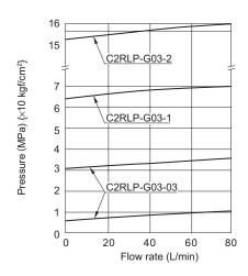
Minimum adjustment pressure characteristics
